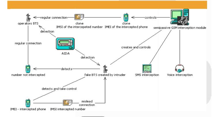
Aida is detecting semi-active interception in GSM/UMTS band and thus identifying malicious BTS in the monitored location that are not part of the arsenal of legally authorised BTS. AIDA monitors the BTS of all the operators and detects any illegal device in the range.
